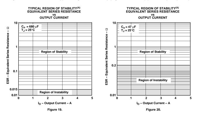
A. Equivalent series resistance (ESR) refers to the total series resistance, including the ESR of the capacitor, any series resistance added externally, and PWB trace resistance to  $C_{\rm O}$ .
