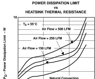
$R_{\theta SA}$  – Heatsink Thermal Resistance –  $^{\circ}\text{C/W}$
