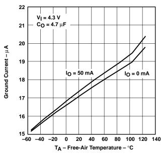
load current (TPS77050) — and is directly proportional to the load current. Since the PMOS pass element is a voltage-driven device, the quiescent current is ultralow (28  $\mu$ A maximum) and is stable over the entire range of output load current (0 mA to 50 mA). Intended for use in portable systems such as laptops and cellular phones, the ultralow-dropout voltage feature and ultralow-power operation result in a significant increase in system battery operating life.
