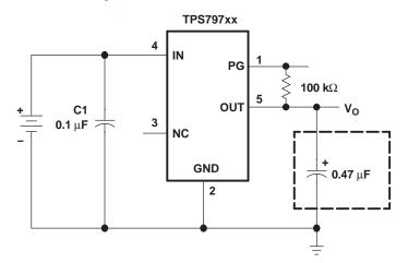
Figure 14. Typical Application Circuit
