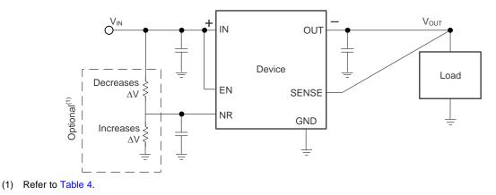
Figure 21. Basic Circuit Connections
