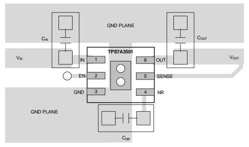
Figure 25. PCB Layout Example (DRV Package)
