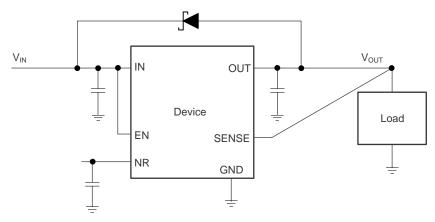
Figure 20. Reverse Current Protection Schematic
