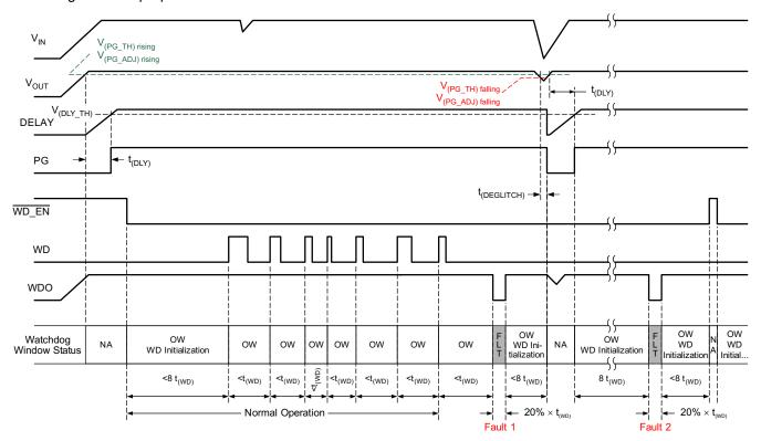
Figure 7-5. Standard Watchdog Operation
