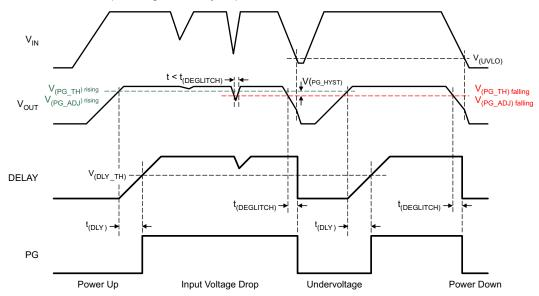
Figure 7-2. Power Up and Conditions for Activating Power-Good
