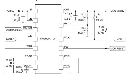
Figure 8-1. TPS7B63xx-Q1 Typical Application Schematic
