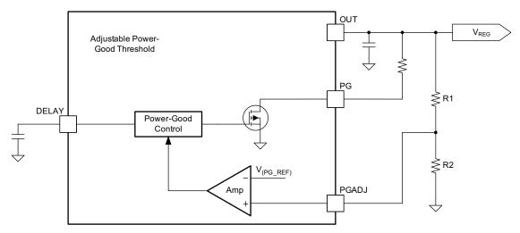
Figure 7-1. Adjustable Power-Good Threshold
