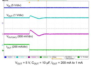
Figure 6-20. Load Transient
