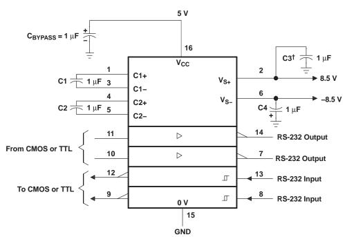
$<sup>^{\</sup>dagger}$  C3 can be connected to  $V_{CC}$  or GND.
