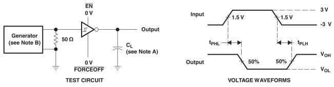
A.C<sub>L</sub> includes probe and jig capacitance.
