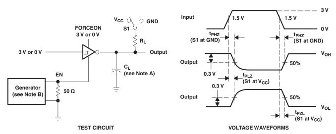
A.C<sub>L</sub> includes probe and jig capacitance.
