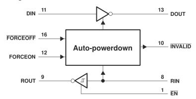
Figure 8-1. Logic Diagram (Positive Logic)
