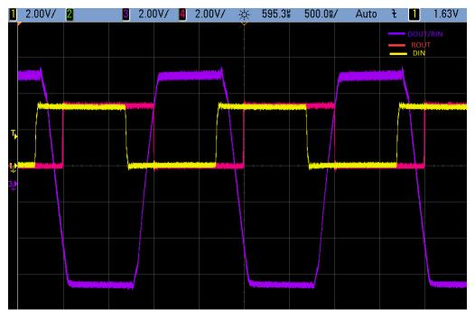
Figure 9-2. 1 Mbps Driver to Receiver Loopback Timing Waveform, V<sub>CC</sub> = 3.3 V
