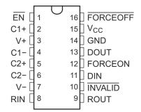
DB or PW Package. 16 Pins (Top View)
