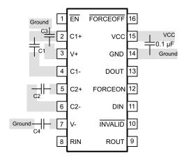
Figure 11-1. Layout Diagram
