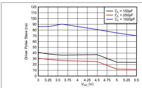
Figure 6-1. Driver Pulse Skew vs Load Capacitance and Supply Voltage at  $T_{\Delta}$  = 25 °C (RGT Package)
