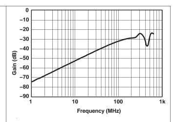
Figure 14. OFF Isolation vs Frequency  $(V_+ = 3.3 \text{ V})$
