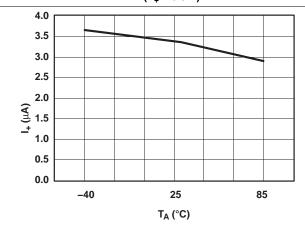
Figure 16. Power-Supply Current vs Temperature  $(V_+ = 3.3 \text{ V})$
