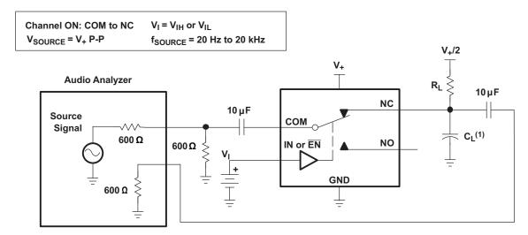
(1)  $C_L$  includes probe and jig capacitance.
