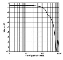
Figure 29. Gain vs Frequency Bandwidth (V<sub>+</sub> = 1.8 V)
