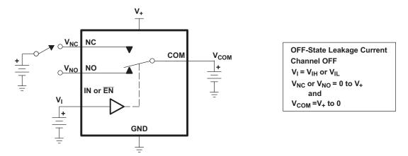
Figure 18. OFF-State Leakage Current ( $I_{COM(OFF)}$ ,  $I_{NC(OFF)}$ ,  $I_{NO(OFF)}$ )
