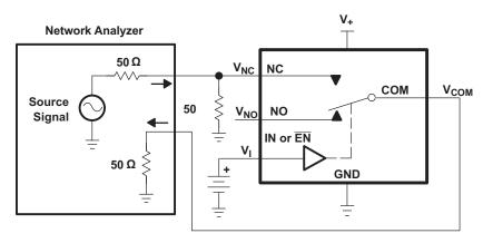
Channel OFF: NC to COM  $V_I = V_+$  or GND
