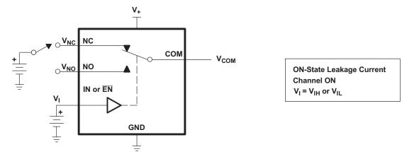
Figure 19. ON-State Leakage Current ( $I_{COM(ON)}$ ,  $I_{NC(ON)}$ )
