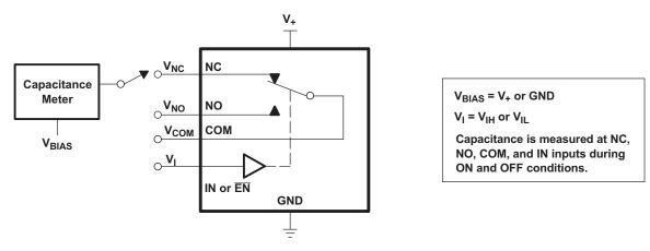
Figure 20. Capacitance (C<sub>I</sub>,  $C_{COM(OFF)}$ ,  $C_{COM(ON)}$ ,  $C_{NC(OFF)}$ ,  $C_{NC(ON)}$ )
