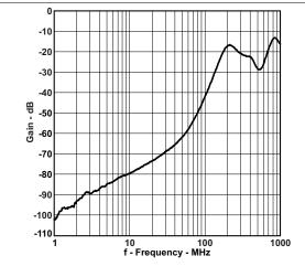
Figure 11. OFF Isolation vs Frequency  $(V_+ = 1.8 \text{ V})$
