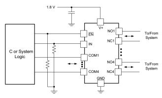
Figure 28. System Schematic for TS3A5018
