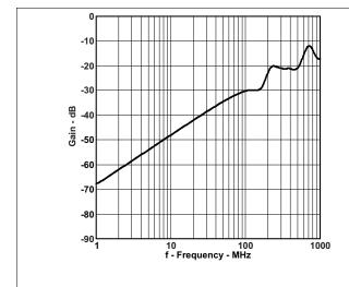
Figure 13. Crosstalk vs Frequency (V<sub>+</sub> = 1.8 V)
