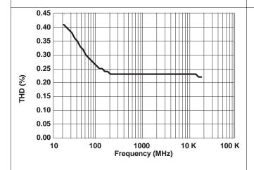
Figure 15. Total Harmonic Distortion vs Frequency
