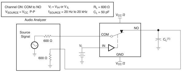
(1) C<sub>L</sub> includes probe and jig capacitance.
