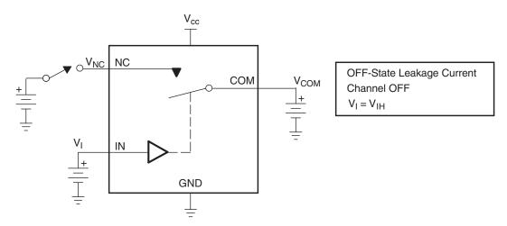
Figure 14. OFF-State Leakage Current (I<sub>COM(OFF)</sub>, I<sub>NC(OFF)</sub>, I<sub>COM(PWROFF)</sub>, I<sub>NC(PWROFF)</sub>)
