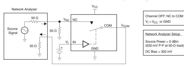
Figure 19. OFF Isolation (O<sub>ISO</sub>)
