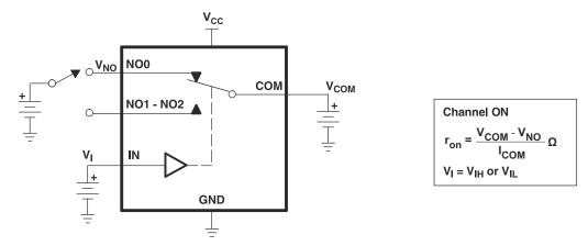
Figure 7-1. ON-State Resistance (R<sub>on</sub>)
