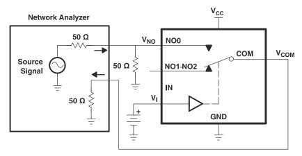
Channel OFF: NO0 to COM V<sub>I</sub> = V<sub>CC</sub> or GND
