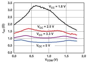
Figure 9-2. Ron vs V<sub>COM</sub>
