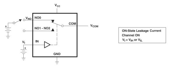
Figure 7-3. ON-State Leakage Current ( $I_{COM(ON)}$ ,  $I_{NO(ON)}$ )
