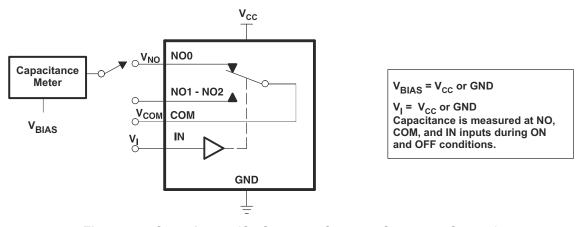
Figure 7-4. Capacitance (C<sub>I</sub>,  $C_{COM(ON)}$ ,  $C_{NO(OFF)}$ ,  $C_{COM(OFF)}$ ,  $C_{NO(ON)}$ )
