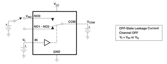
$\textbf{Figure 7-2. OFF-State Leakage Current (I}_{NC(OFF)}, I_{NO(OFF)}, I_{NO(PWROFF)}, I_{COM(PWROFF)})\\$
