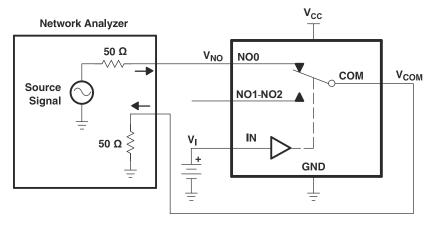
Channel ON: NO0 to COM  $V_I = V_{CC}$  or GND
