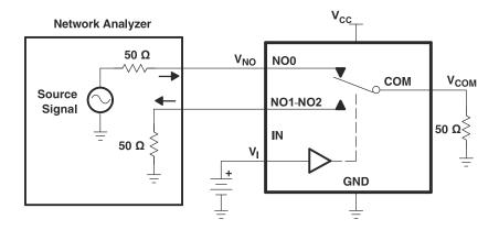
Channel ON: NO0 to COM Channel OFF: NO0-NO1 to COM
