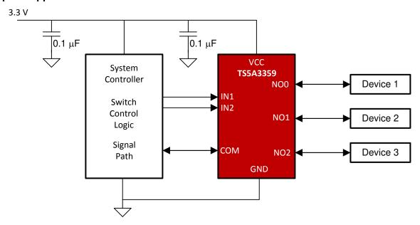
Figure 9-1. Typical Application Schematic
