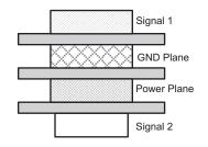
Figure 20. Four-Layer Board Stack-Up
