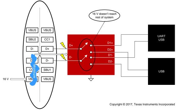
Figure 15. Protecting During a 16-V Short
