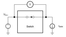
Channel ON,  $R_{ON} = V/I_{SINK}$
