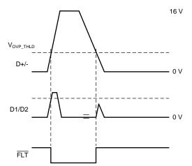
Figure 16. Overvoltage Protection Waveform, 16 V
