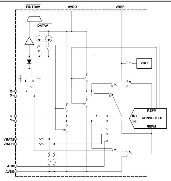
Figure 17. Simplified Diagram of the Analog Input Section
