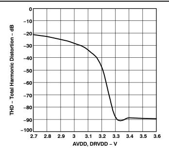
Figure 33. THD vs AVDD, DRVDD Supply Voltage (25°C When Driving a -1 dB, 1-kHz Sinewave From the DAC Into an 8- $\Omega$  Load, with DAC Output Swing Set to 2.4 V, and Short-Circuit Protection Disabled)
