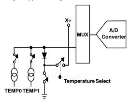
Figure 19. Functional Block Diagram of Temperature Measurement Mode
