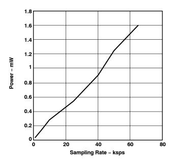
Figure 7. Touch Screen Power Consumption With Speed ( $T_A$  = 25°C, External Ref, Host Controlled AUX Conversion, AVDD = 3.3 V)
