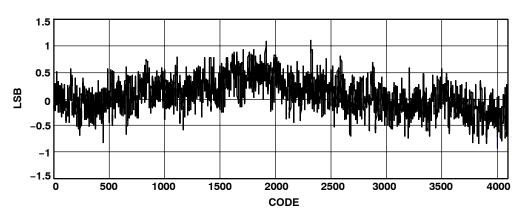
Figure 5. SAR INL ( $T_A = 25$ °C, Internal Ref = 2.5 V, 12 bit, AVDD = 3.3 V)
