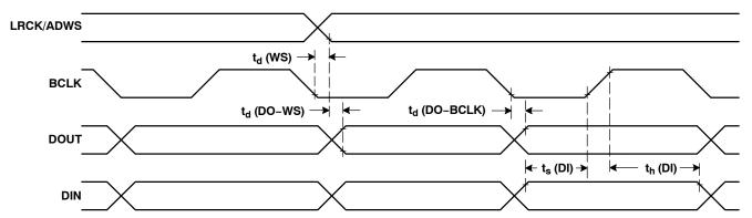
Figure 1. I2S/LJF/RJF Timing in Master Mode
