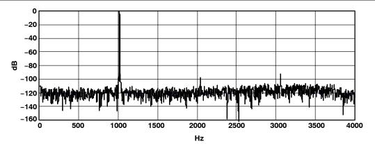
Figure 8. ADC FFT Plot at 8 ksps ( $T_A$  = 25°C, -1 dB, 1 kHz Input, AVDD = 3.3 V)
