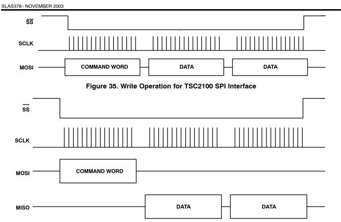
Figure 36. Read Operation for TSC2100 SPI Interface
