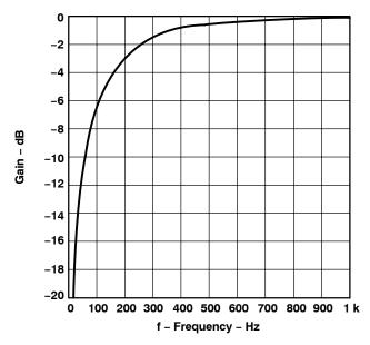
Figure 28. Uncompensated Response For 16- $\Omega$  Load and 50- $\mu$ F Decoupling Capacitor
