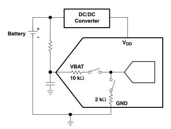
Figure 22. Battery Measurement Functional Block Diagram
