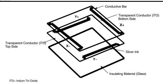
Figure 15. 4-Wire Touch Screen Construction
