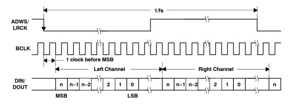
Figure 25. Timing Diagram for I2S Mode
