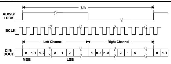
Figure 24. Timing Diagram for Left-Justified Mode
