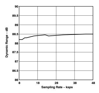
Figure 10. ADC Dynamic Range vs Sampling Speed ( $T_A = 25^{\circ}C$ , AVDD = 3.3 V)
