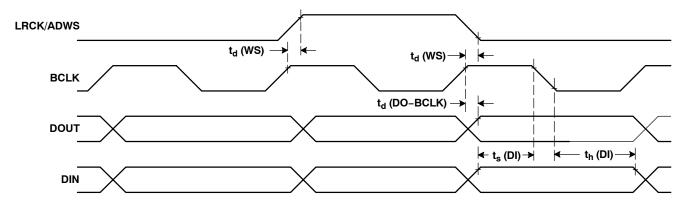
Figure 2. DSP Timing in Master Mode
