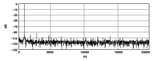
Figure 12. DAC FFT Plot (T<sub>A</sub> = 25°C, 48 ksps, –1 dB, 1 kHz Input, AVDD = DRVDD = 3.3 V, DVDD = 1.8 V, R<sub>L</sub> = 16  $\Omega$ )
