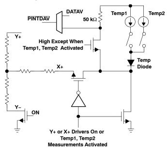
Figure 18. PINTDAV Functional Block Diagram
