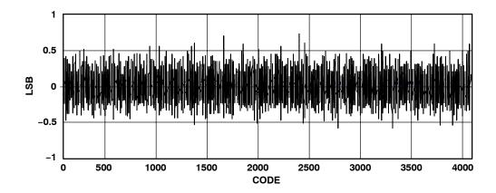
Figure 6. SAR DNL ( $T_A = 25^{\circ}C$ , Internal Ref = 2.5 V, AVDD = 3.3 V)
