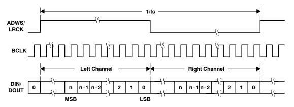
Figure 23. Timing Diagram for Right-Justified Mode
