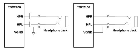
Figure 30. Headphone Configurations, AC-Coupled (left) and Capless (right)
