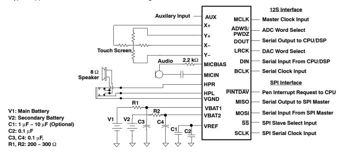
Figure 14. Typical Circuit Configuration
