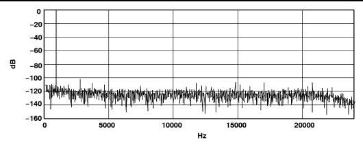
Figure 11. DAC FFT Plot ( $T_A$  = 25°C, 48 ksps, 0 dB, 1 kHz Input, AVDD = 3.3 V,  $R_L$  = 10 k $\Omega$ )
