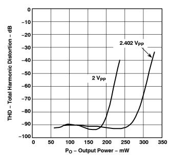
Figure 32. THD vs Output Power Delivered to an an 8-Ω Load (25°C, AVDD = DRVDD = 3.3 V, DVDD = 1.8 V, DAC Output Swing Set to 2 V and 2.4V, and Short-Circuit Protection Disabled)
