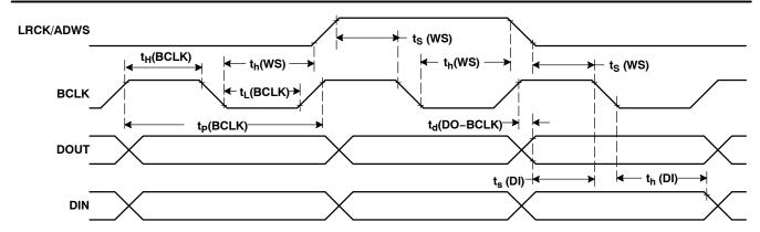
Figure 4. DSP Timing in Slave Mode
