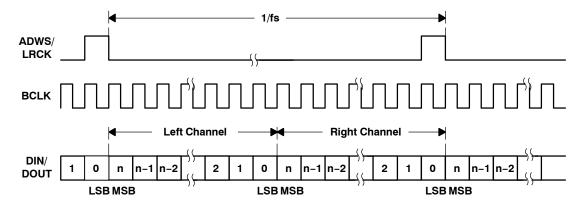
Figure 26. Timing Diagram for DSP Mode
