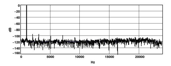
Figure 9. ADC FFT Plot at 48 ksps ( $T_A = 25^{\circ}C$ , -1 dB, 1 kHz Input, AVDD = 3.3 V)
