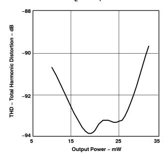
Figure 13. High Power Output Driver THD vs Output Power (T\_A =25°C, AVDD, DRVDD = 3.3 V, R\_L = 16  $\Omega$ )
