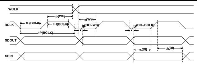
Figure 3. I<sup>2</sup>S/LJF/RJF Timing in Slave Mode
