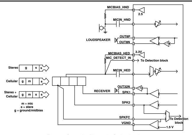
Figure 22. Connection Diagram for Capless Interface
