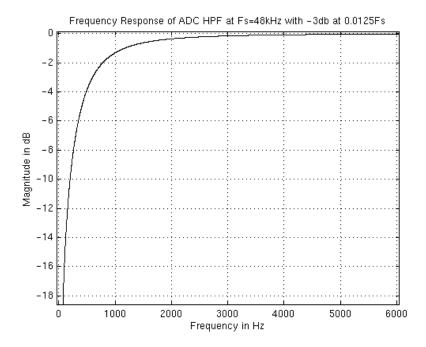
Figure 41. Frequency Response of ADC High-Pass Filter (Fcutoff = 0.0125 Fs)
