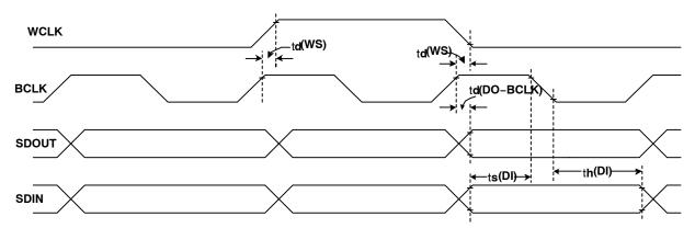
Figure 2. DSP Timing in Master Mode
