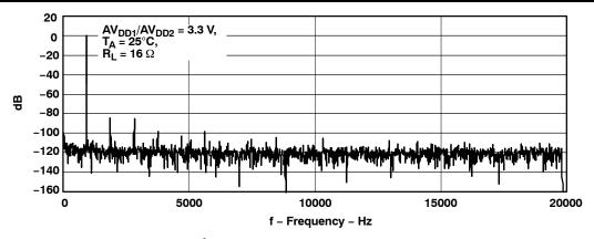
Figure 11. DAC FFT Plot ( $T_A$  = 25 $^{\circ}$ C, -1 dB, 1 kHz Input, AVDD1/AVDD2/DRVDD = 3.3 V,  $R_L$  = 16  $\Omega$ )
