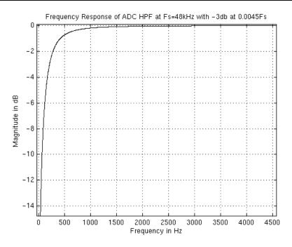
Figure 40. Frequency Response of ADC High-Pass Filter (Fcutoff = 0.0045 Fs)
