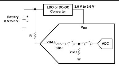
Figure 33. Battery Measurement Functional Block Diagram
