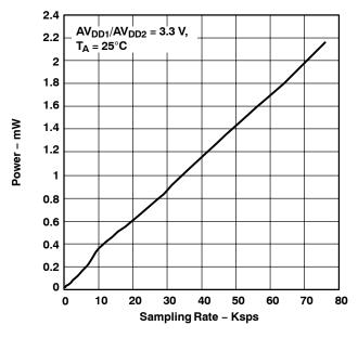
Figure 7. SAR ADC Power Consumption vs Speed ( $T_A = 25^{\circ}C$ , External Reference, Host Controlled AUX Conversion, AVDD1/AVDD2 = 3.3 V)
