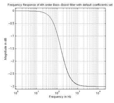
Figure 45. Default Digital Audio Effects Filter Frequency Response at 48 Ksps
