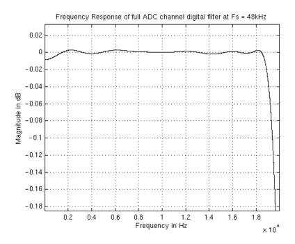
Figure 39. Pass-Band Frequency Response of ADC Digital Filter
