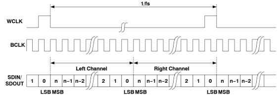
Figure 18. Timing Diagram for DSP Mode
