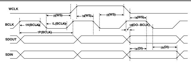
Figure 4. DSP Timing in Slave Mode
