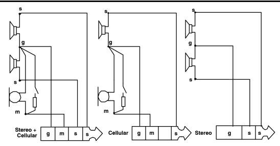
Figure 24. Connection Diagram for Jacks
