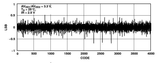
Figure 6. SAR DNL ( $T_A = 25^{\circ}C$ , Internal Reference = 2.5 V, 12 bit, AVDD1/AVDD2 = 3.3 V)
