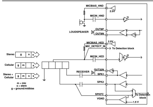
Figure 23. Connection Diagram for Cap Interface
