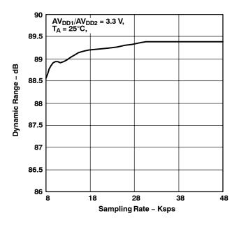
Figure 10. ADC Dynamic Range vs Sampling Rate (T<sub>A</sub> = 25°C, AVDD1/AVDD2 = 3.3 V)
