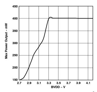
Figure 14. Loudspeaker Driver Output Power vs BVDD (T<sub>A</sub> = 25 $^{\circ}$ C, 1 kHz Input, AVDD1/AVDD2/DRVDD = 3.3 V, R<sub>L</sub> = 8  $\Omega$ , THD  $\leq$  -40 dB)
