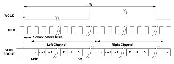
Figure 17. Timing Diagram for I2S Mode
