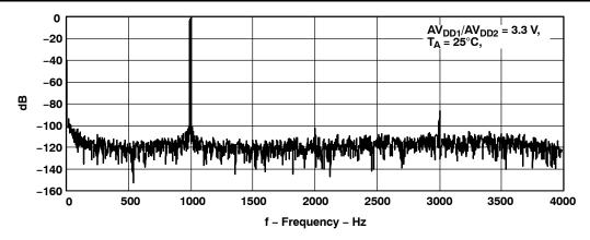
Figure 8. ADC FFT Plot at 8 ksps ( $T_A = 25^{\circ}C$ , -1 dB, 1 kHz input, AVDD1/AVDD2 = 3.3 V)
