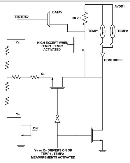
Figure 28. PINTDAV Functional Block Diagram
