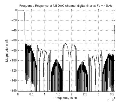
Figure 43. DAC Channel Digital Filter Frequency Response
