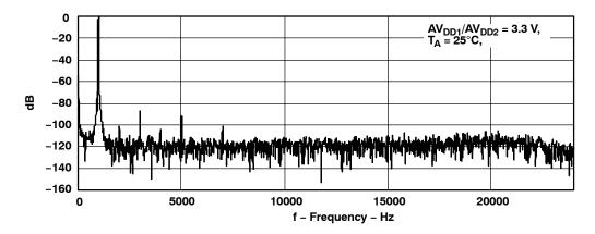
Figure 9. ADC FFT Plot at 48 ksps ( $T_A = 25^{\circ}C$ , -1 dB, 1 kHz input, AVDD1/AVDD2 = 3.3 V)
