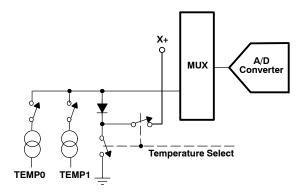
Figure 29. Functional Block Diagram of Temperature Measurement Mode
