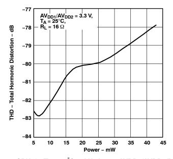
Figure 12. THD vs Power on SPK1/2 ( $T_A$  = 25 $^{\circ}$ C, 1 kHz Input, AVDD1/AVDD2/DRVDD = 3.3 V,  $R_L$  = 16  $\Omega$ )
