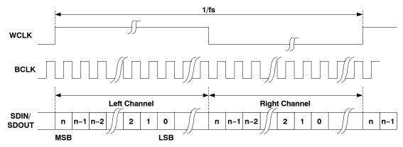
Figure 16. Timing Diagram for Left-Justified Mode
