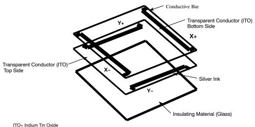
Figure 25. 4-Wire Touch Screen Construction
