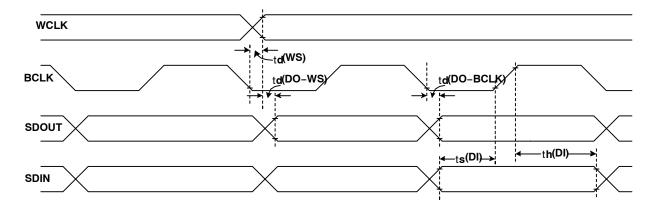
Figure 1. I2S/LJ/RJ in Master Mode
