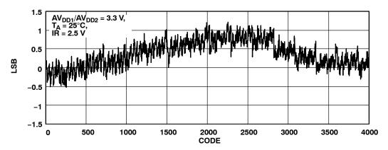
Figure 5. SAR INL (T<sub>A</sub> = 25°C, Internal Reference = 2.5 V, 12 bit, AVDD1/AVDD2 = 3.3 V)
