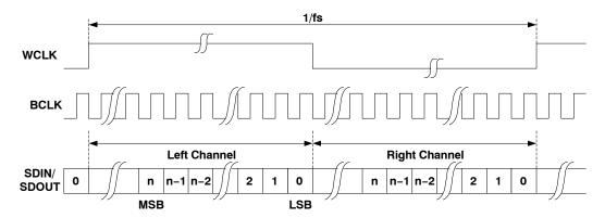
Figure 15. Timing Diagram for Right-Justified Mode
