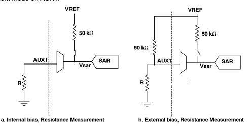
Figure 34. Connection Diagram for Resistance Measurement
