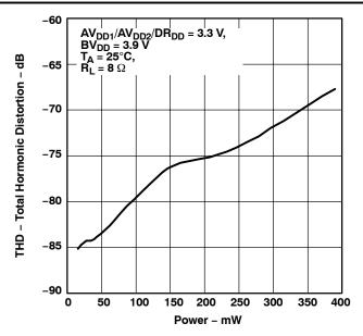
Figure 13. THD vs Power on Loudspeaker Driver (T<sub>A</sub> = 25 $^{\circ}$ C, 1 kHz Input, AVDD1/AVDD2/DRVDD = 3.3 V, BVDD = 3.9 V, R<sub>L</sub> = 8  $\Omega$ )
