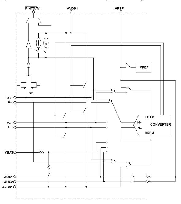
Figure 27. Simplified Diagram of the Analog Input Section
