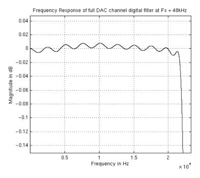
Figure 44. DAC Channel Digital Filter Pass-Band Frequency Response
