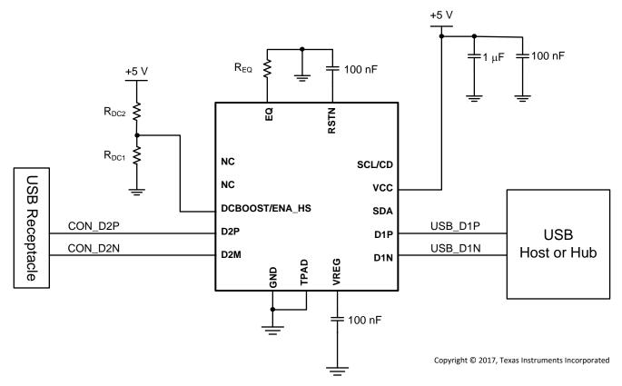
Figure 7. Reference Schematic
