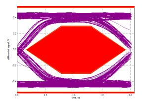
Figure 5. USB2.0 HS Eye diagram, Host far-end with 5m cable pre-channel loss with TUSB213-Q1
