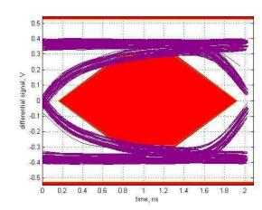
Figure 2. USB2.0 HS Eye diagram, Host far-end with 2m cable post-channel loss without TUSB213-Q1
