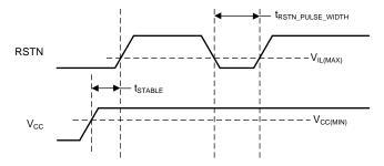
Figure 1. Power On and Reset Timing
