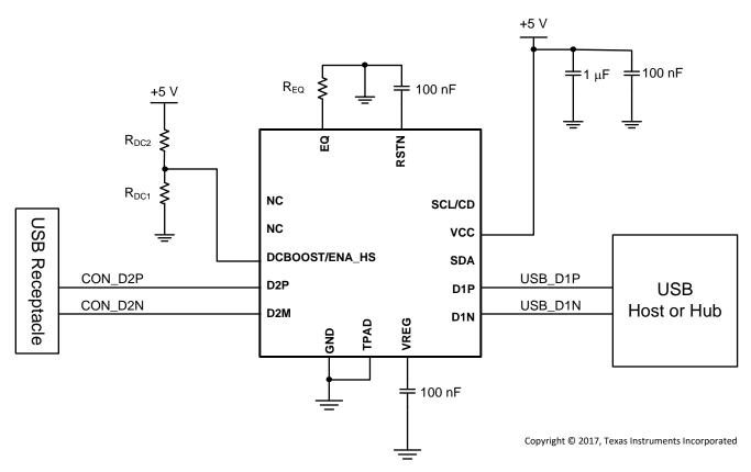
Figure 7. Reference Schematic
