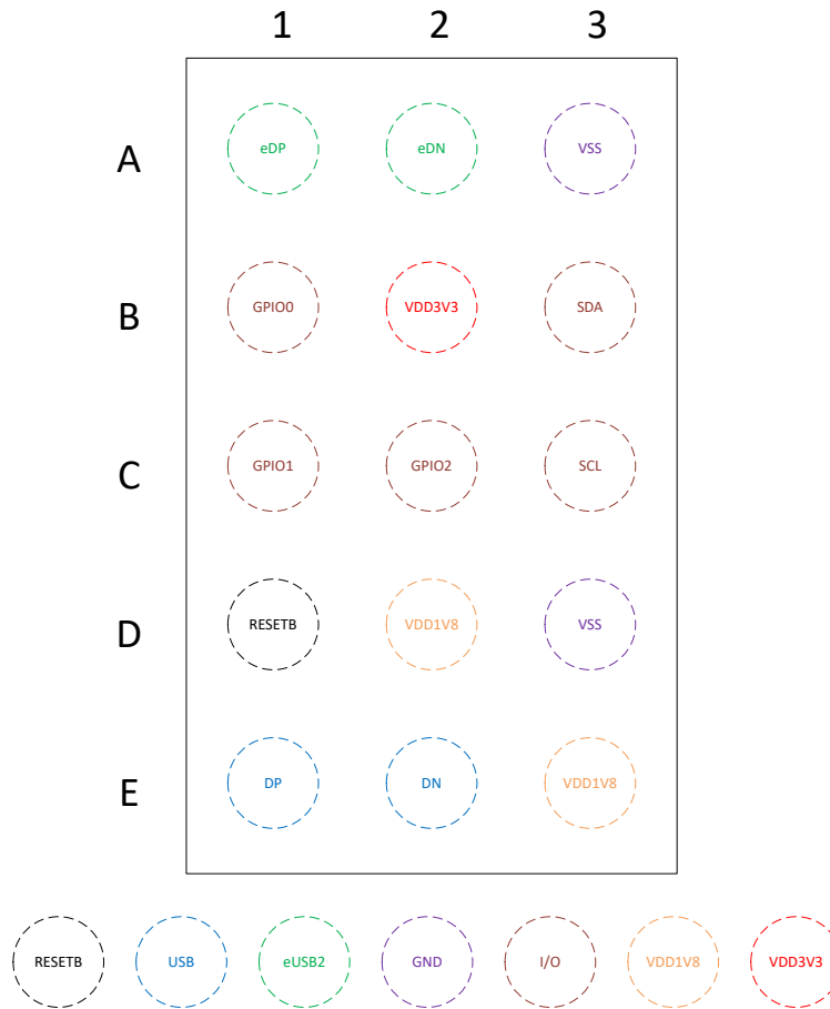
Figure 6-1. TUSB2E11 YCG Package, 15-Pin DSBGA (Top View)
