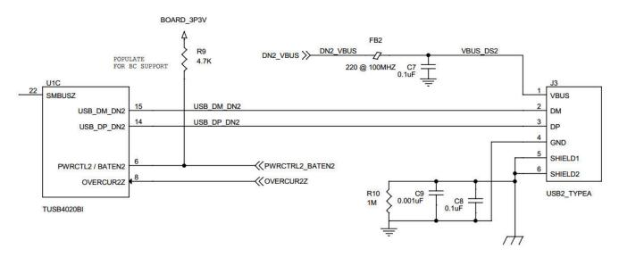
Figure 9-6. Downstream Port 2 Implementation Schematic
