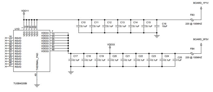
Figure 9-9. Power Implementation Schematic
