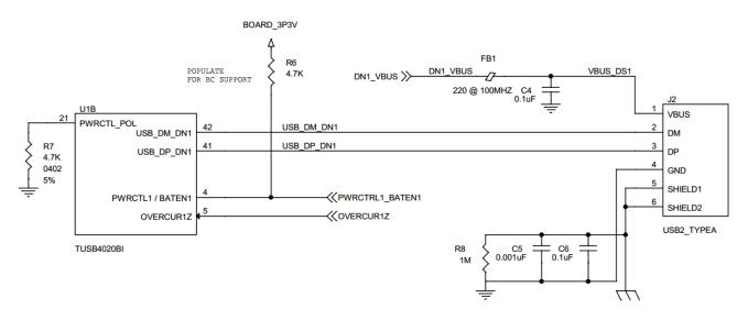
Figure 9-5. Downstream Port 1 Implementation Schematic
