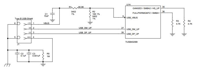
Figure 9-2. Upstream Port Implementation Schematic
