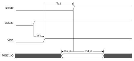
Figure 7-1. Power-Up Timing Requirements
