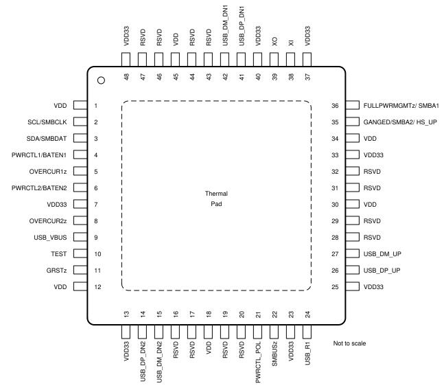
Figure 6-1. PHP Package 48-Pin HTQFP Top View
