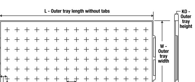
P1 - Tray unit pocket pitch CW - Measurement for tray edge (Y direction) to corner pocket center - CL - Measurement for tray edge (X direction) to corner pocket center
