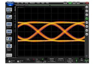
Figure 21. Output Signal: 24 Inch Output Trace (Eye Diagram at the DCAX)
