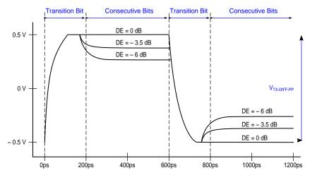
Figure 14. Transmitter Differential Voltage in Presence of De-Emphasis
