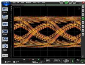
Figure 20. Input Signal: 24 Inch Input Trace (Eye Diagram at the Re-driver input)
