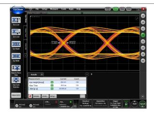
Figure 12. Output Signal: 24-Inches Output Trace
