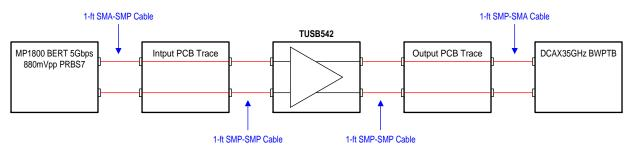
Figure 17. Measurement Setup
