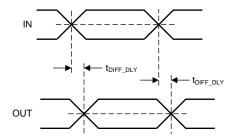
Figure 1. Propagation Delay Timing
