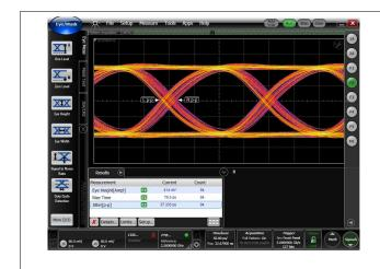
Figure 11. Output Signal: 12-Inches Output Trace
