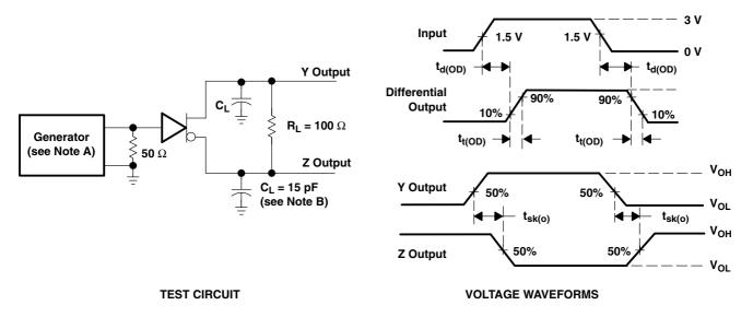
NOTES: A. The input pulse generator has the following characteristics:  $Z_O$  = 50  $\Omega$ , PRR  $\leq$  500 kHz,  $t_w$  = 100 ns,  $t_r$  =  $\leq$  5 ns.
