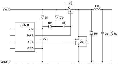
Figure 11. Synchronous Rectifier Application With Charge Pump to Drive High-Side N-Channel Buck Switch. V<sub>IN</sub> is Limited to 10 V as V<sub>CC</sub> Will Rise to Approximately 2V<sub>IN</sub>
