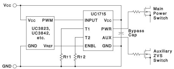
Figure 7. Typical Application With Timed Delays
