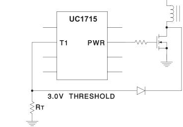
Figure 8. Using the Timer Input for Zero-Voltage Sensing
