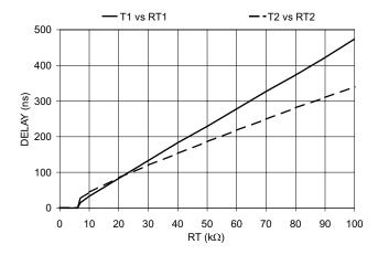
Figure 2. T1 Delay, T2 Delay vs.  $R_{\mathsf{T}}$
