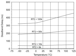
Figure 6. T2 Deadband vs. Temperature PWR to AUX
