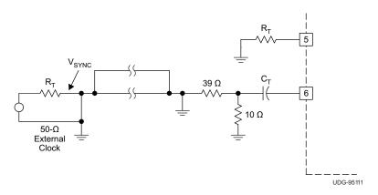
Figure 8. General Oscillator Synchronization
