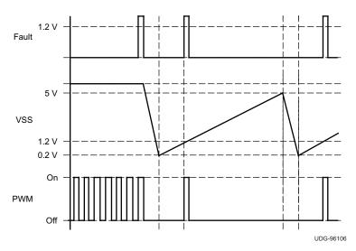
Figure 4. Soft-Start and Fault Waveforms
