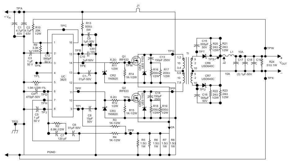
Figure 16. Typical Application Schematic
