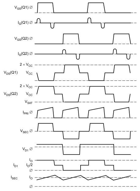
Figure 24. Basic Push-Pull Waveforms
