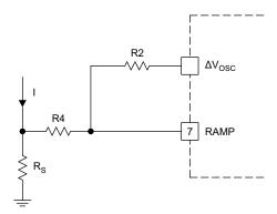
Figure 21. Slope Compensation Steps
