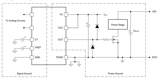
Figure 25. Ground Planes Diagram
