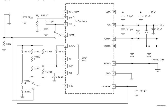
Figure 12. Open Loop Test Circuit Schematic
