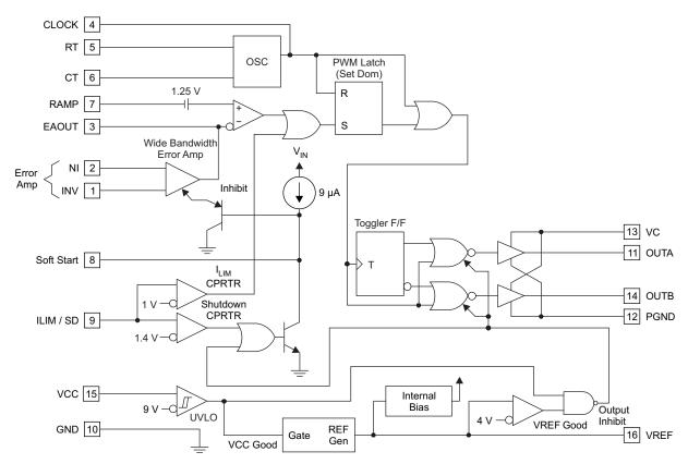
Figure 23. UC1825A-SP Block Diagram
