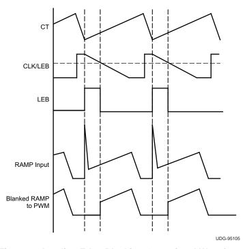
Figure 3. Leading Edge Blanking Operational Waveforms
