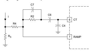
Figure 20. Slope Compensation Steps
