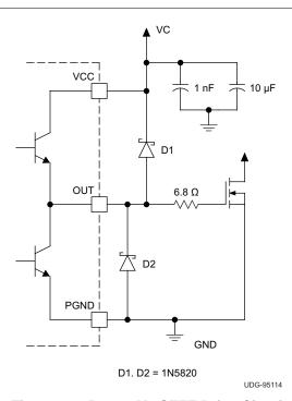
Figure 11. Power MOSFET Drive Circuit
