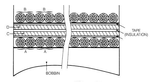
Figure 19. Transformer - Exploded View
