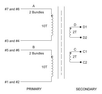
Figure 18. Transformer Schematic
