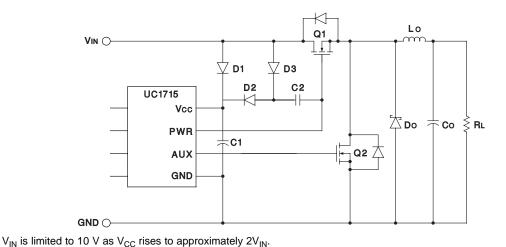
Figure 11. Synchronous Rectifier Application With A Charge Pump To Drive The High-Side N-Channel Buck Switch
