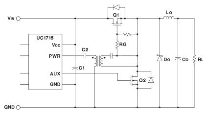
Figure 10. Using The UC1715 As A Complementary Synchronous Rectifier Switch Driver With N-Channel FETs
