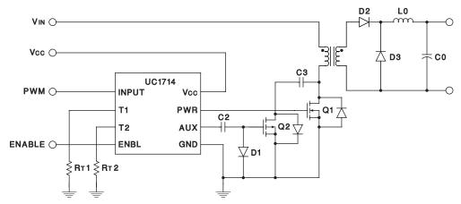
With active reset provided by the UC1714 driving an N-channel switch (Q1) and a P-channel auxiliary switch (Q2).
