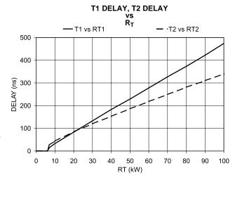
(2) T1 delay is defined from the 50% point of the transition edge of AUX to the 10% of the rising edge of PWR. T2 delay is defined from the 90% of the falling edge of PWR to the 50% point of the transition edge of AUX.
