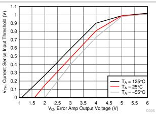
Figure 7-2. Current Sense Input Threshold vs Error Amplifier
