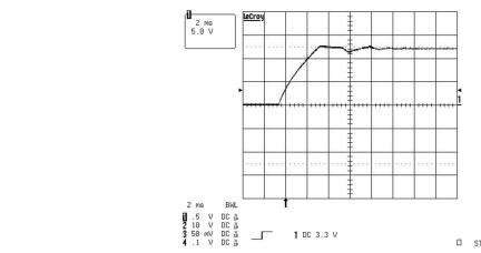
Figure 9-11. Output Voltage Behavior at Full Load Start-Up (5 V/div)
