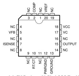
Figure 6-3. FK Package 20-Pin LCCC Top View
