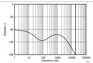
Figure 9-6. Converter Closed-Loop Bode Plot – Phase
