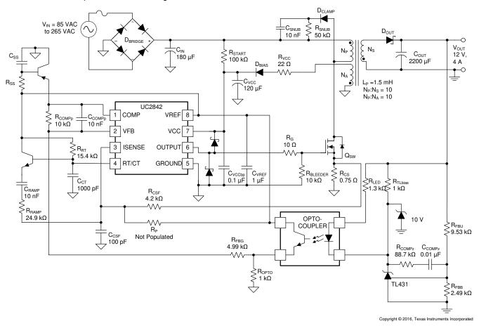
Figure 9-2. Typical Application Design Example Schematic
