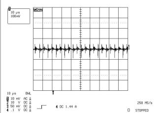
Figure 9-10. Output Voltage Ripple at Full Load (100 mV/div)
