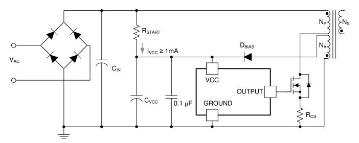
Figure 8-7. Providing Power to UCx84x
