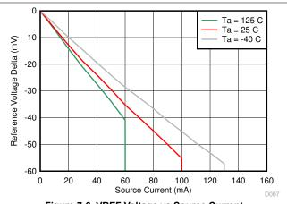
Figure 7-6. VREF Voltage vs Source Current
