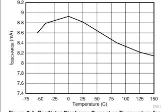
Figure 7-1. Oscillator Discharge Current vs Temperature for VCC = 15 V and V<sub>OSC</sub> = 2 V
