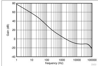
Figure 9-5. Converter Closed-Loop Bode Plot – Gain
