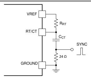
Figure 8-9. Synchronizing the Oscillator
