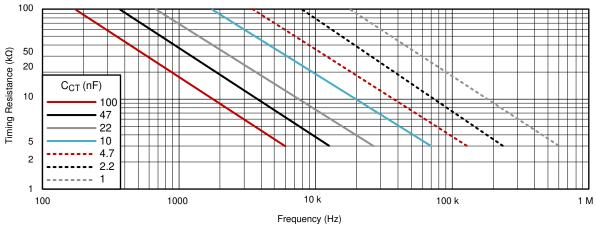
Figure 7-10. Timing Resistance, R<sub>RT</sub>, vs Frequency
