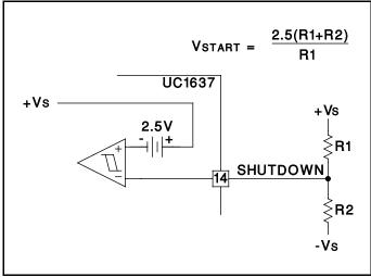
Figure 4. External Under-Voltage Lockout
