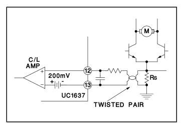
Figure 6. Current Limit Sensing
