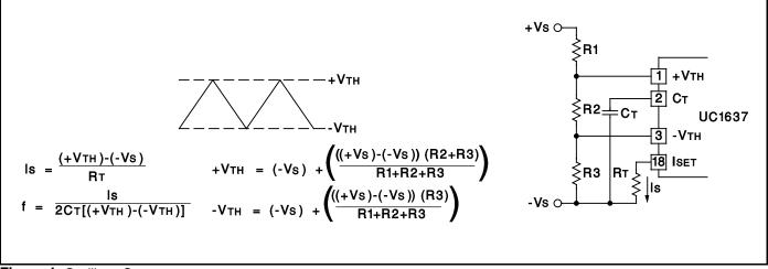
Figure 1. Oscillator Setup
