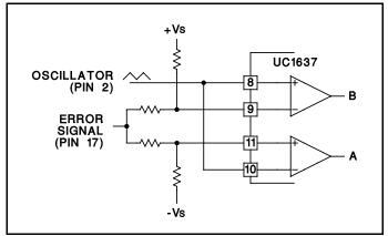
Figure 2. Comparator Biasing
