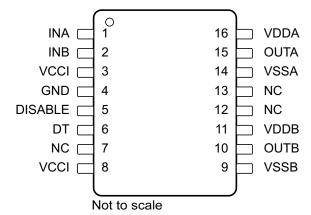
Figure 6-1. DW Package 16-Pin SOIC Top View
