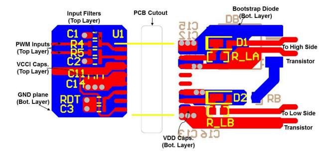
Figure 12-1 shows a 2-layer PCB layout example with the signals and key components labeled.
