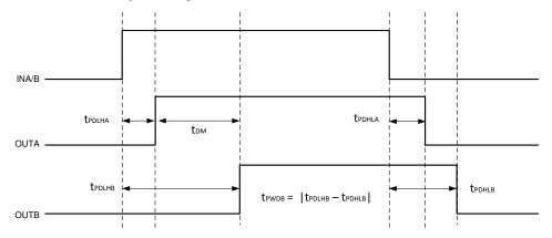
Figure 8-1. Overlapping Inputs, Dead Time Disabled
