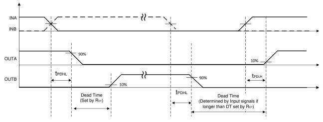
Figure 8-4. Dead-Time Switching Parameters
