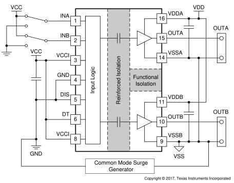
Figure 8-7. Simplified CMTI Testing Setup
