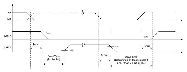
Figure 7-4. Dead-Time Switching Parameters
