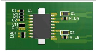
Figure 11-4. 3-D PCB Top View
