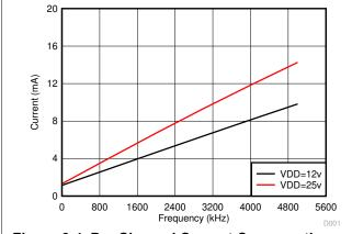
Figure 6-4. Per Channel Current Consumption vs. Frequency (No Load, VDD = 12 V or 25 V)
