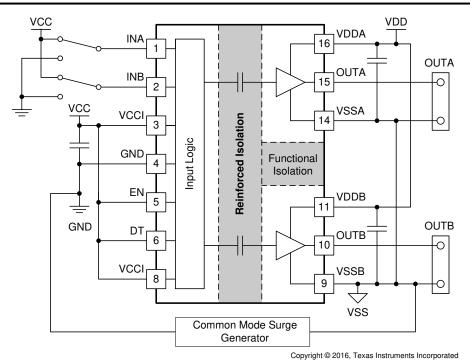
Figure 7-7. Simplified CMTI Testing Setup
