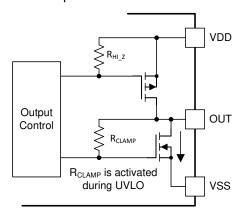
Figure 8-1. Simplified Representation of Active Pulldown Feature
