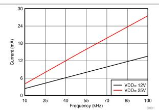
Figure 6-6. Per Channel Current Consumption (I<sub>VDDA/B</sub>) vs. Frequency (10-nF Load, VDD = 12 V or 25 V)
