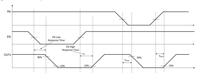
Figure 7-3. Enable Pin Timing
