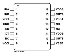
Figure 5-1. DW Package 16-Pin SOIC Top View
