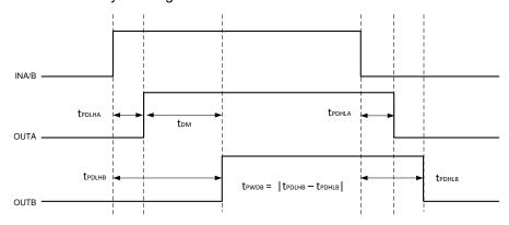
Figure 7-1. Overlapping Inputs, Dead Time Disabled
