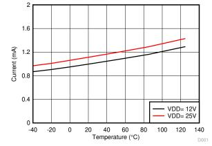
Figure 6-8. Per Channel (I<sub>VDDA/B</sub>) Quiescent Supply Current vs Temperature (No Load, Input Low, No Switching)
