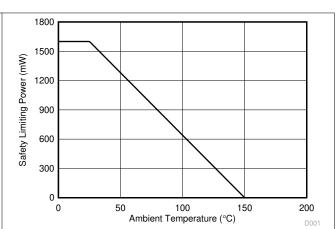
Figure 6-3. Thermal Derating Curve for Safety-Related Limiting Power
