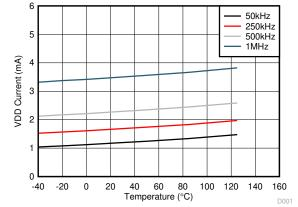
Figure 6-7. Per Channel (I<sub>VDDA/B</sub>) Supply Current Vs. Temperature (VDD=12V, No Load, Different Switching Frequencies)
