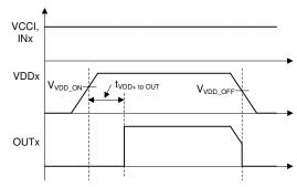
Figure 7-6. VDDA/B Powerup UVLO Delay
