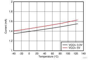
Figure 6-9. I<sub>VCCI</sub> Quiescent Supply Current vs Temperature (No Load, Input Low, No Switching)
