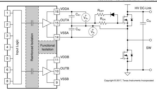
Figure 9-3. Negative Bias with Two Iso-Bias Power Supplies
