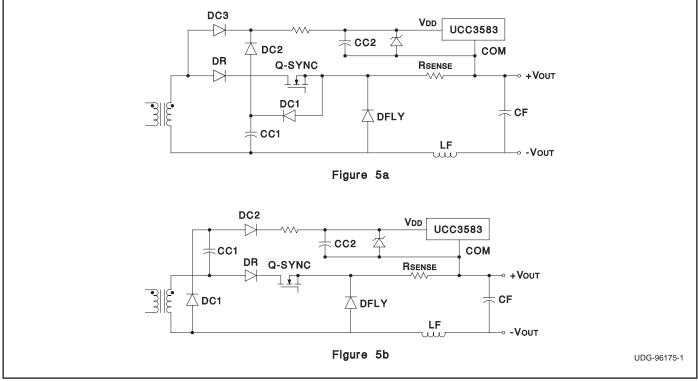
Figure 5. Possible implementation for floating bias voltage generation.
