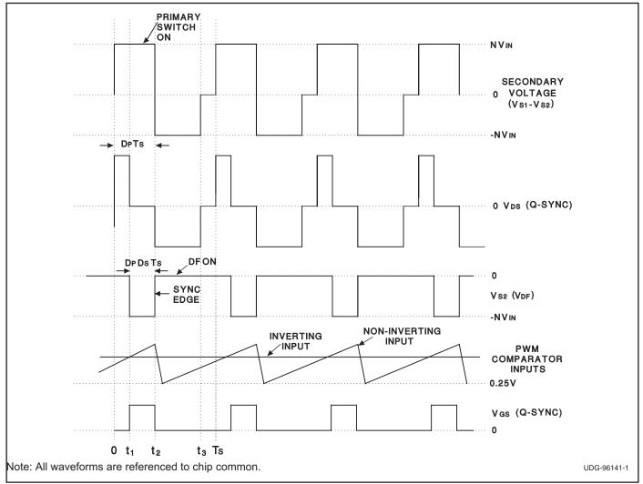
Figure 2. Single ended post regulator waveforms.
