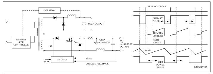
Figure 1. UCC3583 SSPR system application and typical waveforms.
