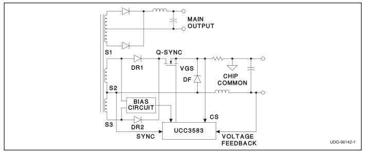
Figure 3. Half-bridge synchronous post regulator application.
