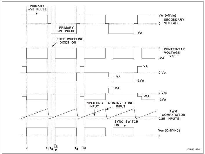
Figure 4. Half-bridge synchronous post regulator to waveforms.
