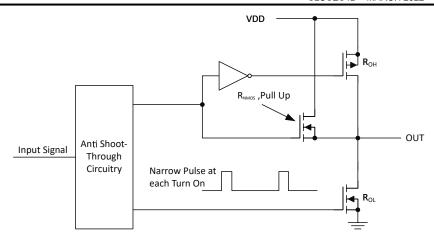
Figure 7-1. UCC27624-Q1 Gate Driver Output Structure
