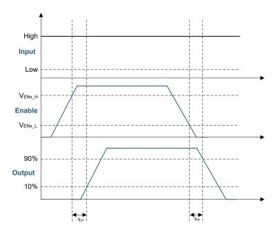
Figure 6-1. Enable Function
