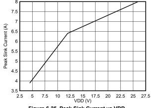
Figure 6-25. Peak Sink Current vs VDD
