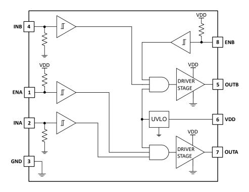
Typical ENx pullup resistance is 200 k $\Omega$  and INx pulldown resistance is 120 k $\Omega$ .
