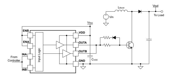
Figure 8-3. UCC27624-Q1 Used to Drive IGBT in the Boost Converter
