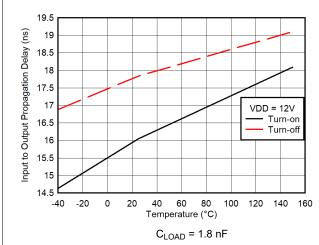
Figure 6-19. Input Propagation Delay vs Temperature
