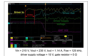
Figure 8-4. Turn-On Propagation Delay Waveform
