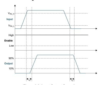
Figure 6-2. Input-Output Operation
