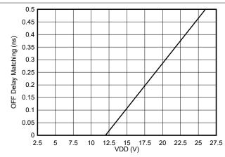
Figure 6-23. Turn-Off and Falling Delay Matching
