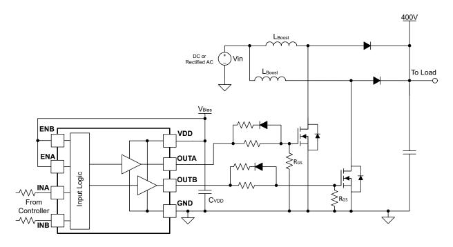
Figure 8-1. UCC27624-Q1 Typical Application Diagram
