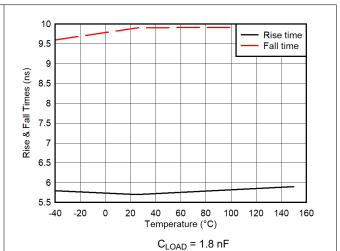
Figure 6-16. Output Rise and Fall Time vs Temperature
