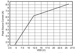
Figure 6-24. Peak Source Current vs VDD
