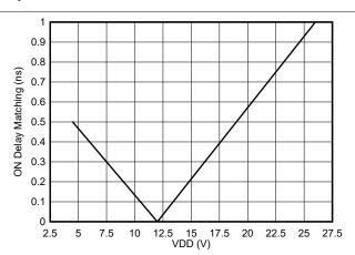
Figure 6-22. Turn-on/Rising Delay Matching
