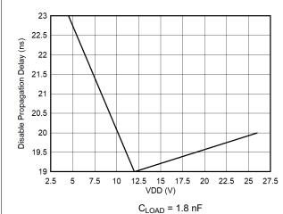
Figure 6-21. Enable to Output Falling Propagation Delay
