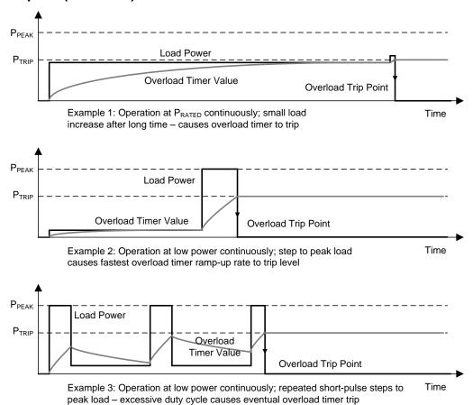
Figure 34. Overload Timer Example Waveforms Under Various Load Scenarios
