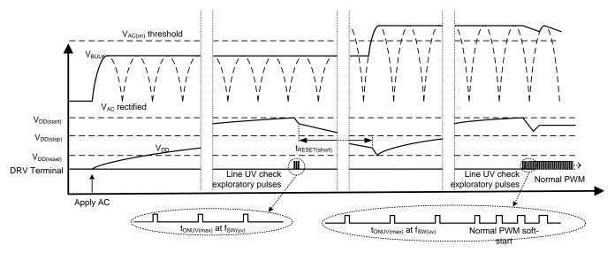
Figure 17. AC Input UVLO Detection and Start Up
