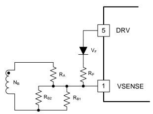
Figure 28. Practical Magnetic Sense Setup with Extra Resistor R<sub>B2</sub> for Setpoint Fine Adjust
