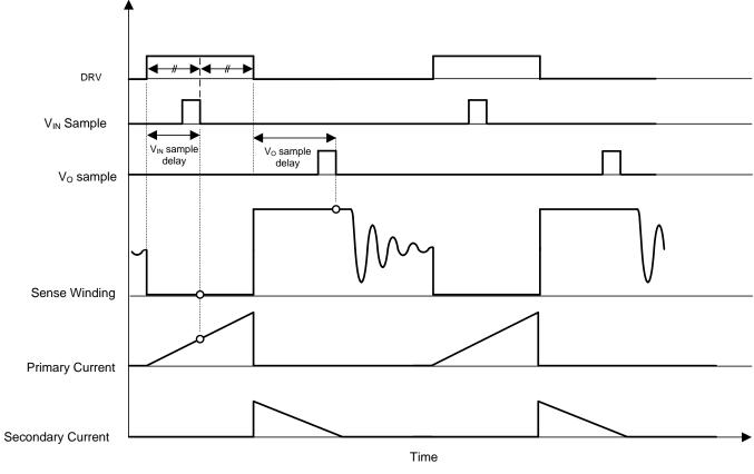
Figure 26. V<sub>IN</sub> and V<sub>OUT</sub> Sample Trigger Timing
