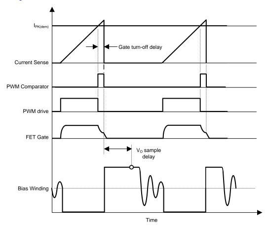
Figure 25. V<sub>OUT</sub> Sample Adjust for External Gate Delay
