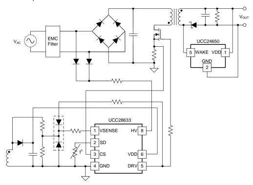
Figure 39. UCC24650 Secondary-Side Voltage Monitor and Wake-Up Circuit
