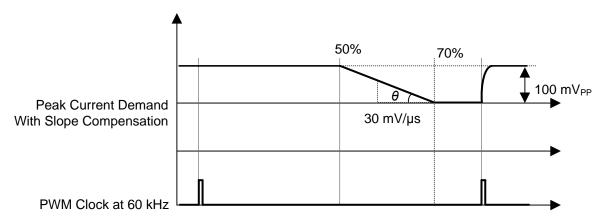
Figure 31. Peak Current Demand with Slope Compensating Downslope
