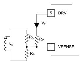
Figure 21. VSENSE Pin Interface Arrangement
