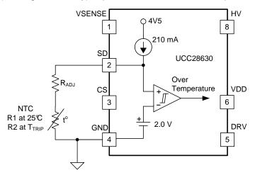
Figure 37. Fault Interface to SD Pin
