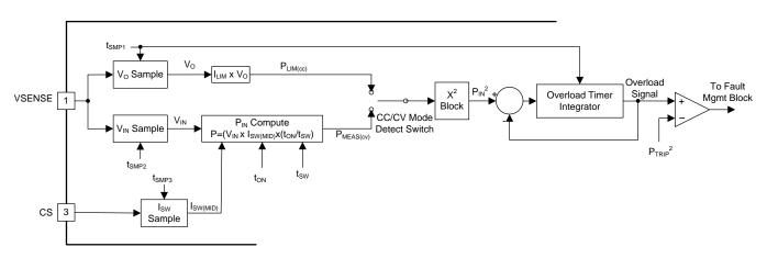
Figure 35. Overload Timer Block Diagram
