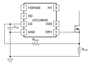
Figure 30. Primary-Side Current Sensing
