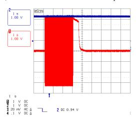
Figure 19. X-Capacitor Discharge Activation, at 230 V<sub>AC</sub>, No Load (red = X-capacitor, blue = bulk-capacitor, both 100 V/div)
