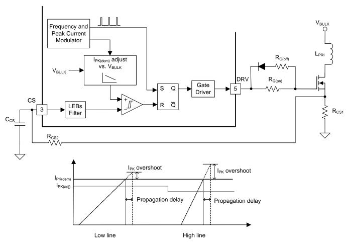
Figure 32. Peak-Current Demand Adjustment vs V<sub>BULK</sub> to Correct Prop Delay Overshoot
