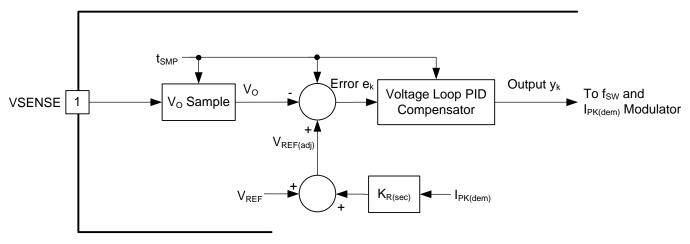
Figure 29. Digital Voltage Control Loop Simplified Block Diagram
