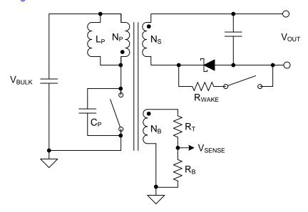
Figure 45. Simplified Equivalent Circuit of Wake Event with UCC24650
