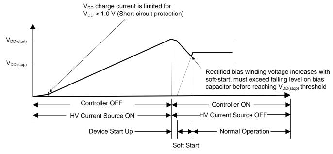
Figure 16. Normal Start-Up Sequence, (assuming  $V_{AC} > UV$  start threshold)
