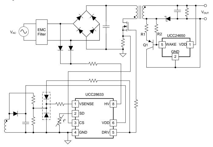
Figure 40. Augmented UCC24650 Secondary-Side Voltage Monitor and Wake-Up Circuit
