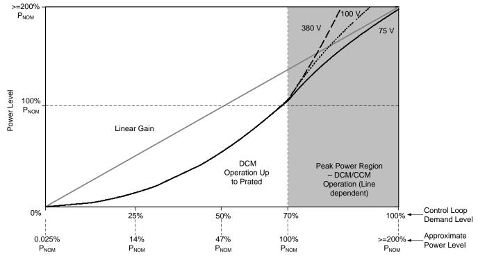
Figure 42. Modulator Gain Curves vs Bulk Capacitor Voltage
