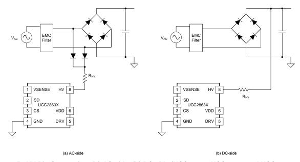
Figure 15. HV Pin Connection: (a) AC-side, (b) DC-side (UCC28631, UCC28632 and UCC28634 only)
