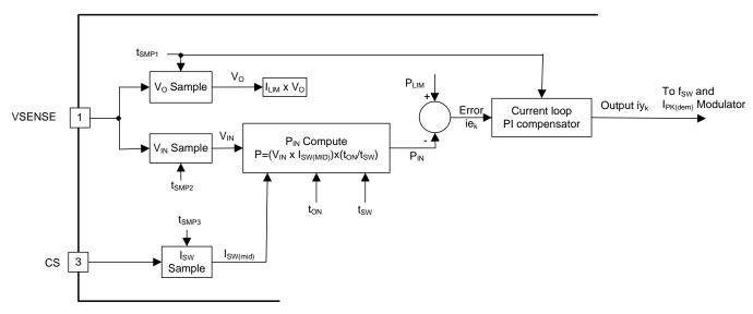
Figure 33. Digital Current Control Loop Simplified Block Diagram
