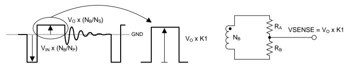
Figure 22. V<sub>OUT</sub> Sense Using the Positive Swing on the Sense Winding
