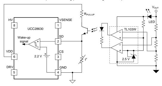
Figure 38. Typical Secondary-Side Voltage Monitor and Wake-Up Circuit for Interfacing to the SD Pin
