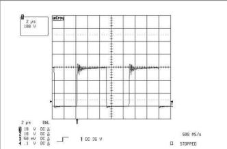
Figure 9-9. Primary Side MOSFET Drain to Source Voltage at 120-V AC Input (100 V/div)
