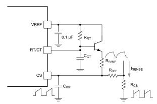
Figure 8-8. Slope Compensation Circuit
