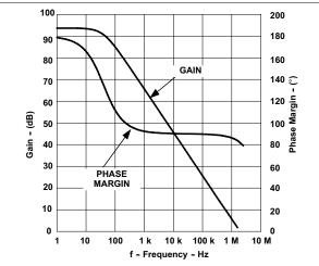
Figure 7-3. Error Amplifier Frequency Response
