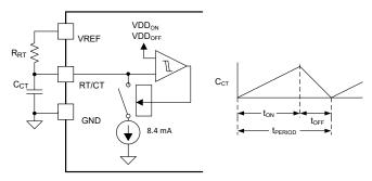
Figure 8-4. Oscillator Circuit
