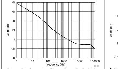
Figure 9-6. Converter Closed-Loop Bode Plot – Gain
