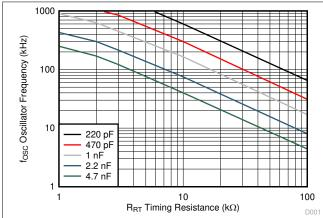
Figure 7-1. Oscillator Frequency vs Timing Resistance and Capacitance
