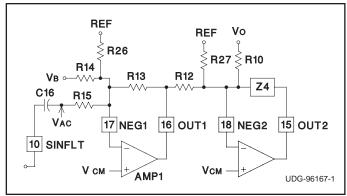
Figure 6. Error amplifier setup.
