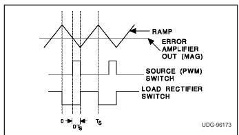
Figure 3. Circuit waveforms.
