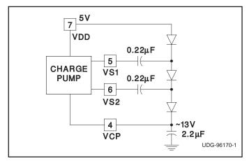
Figure 9. Charge pump circuits.
