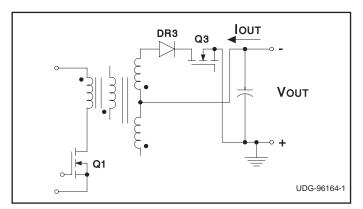
Figure 4c. Mode 3: Forward power transfer, negative output.
