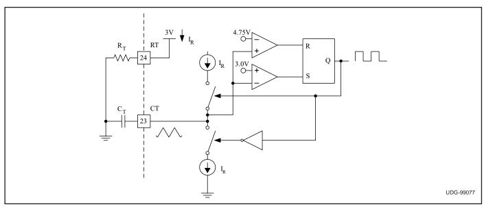
Figure 7. Oscillator setup.
