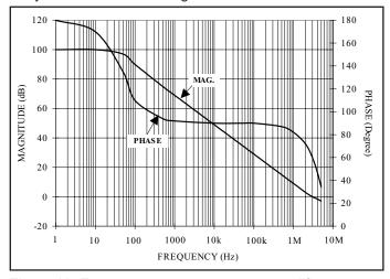
Figure 10. Frequency response to error amplifiers.
