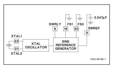
Figure 5. Sine-wave generator.
