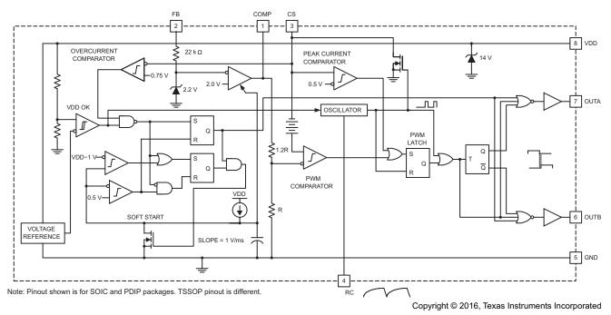
The oscillator generates a sawtooth waveform on RC. During the RC rise time, the output stages alternate on time, but both stages are off during the RC fall time. The output stages switch a 1/2 the oscillator frequency, with ensured duty cycle of < 50% for both outputs.
