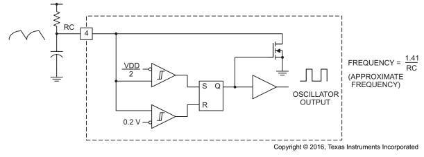
Figure 10. Block Diagram of Oscillator
