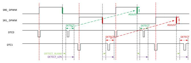
Figure 5-7. Timing Diagram of the DTC Interface
