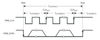
Figure 5-2. Bus Timing in Extended Mode
