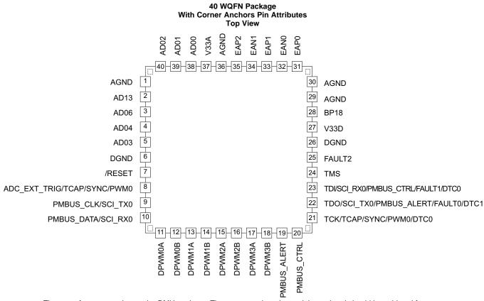
There are four corner pins on the RMH package. The corner anchor pins and thermal pad should be soldered for robust mechanical performance and should be tied to the appropriate ground signal.
