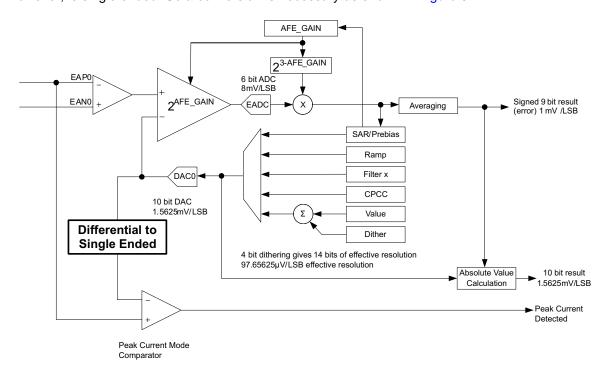
Figure 8-14. Differential to Single-Ended Comparator Function
