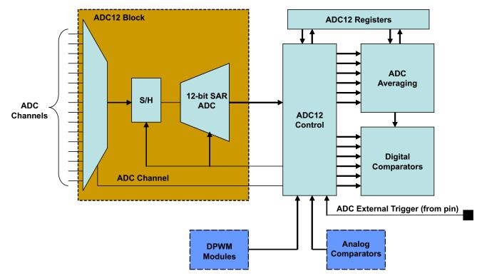
Figure 7-14. ADC12 Control Block Diagram
