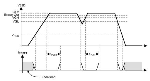
Figure 6-2. Power-On Reset (POR) and Brown-Out Reset (BOR)
