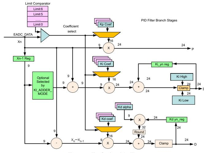
Figure 7-6. First Section of the Filter
