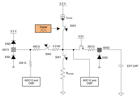
Figure 7-16. Simplified Current Sharing Circuitry
