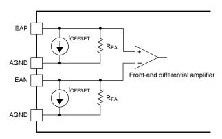
Figure 5-3. Input Stage of EADC Module
