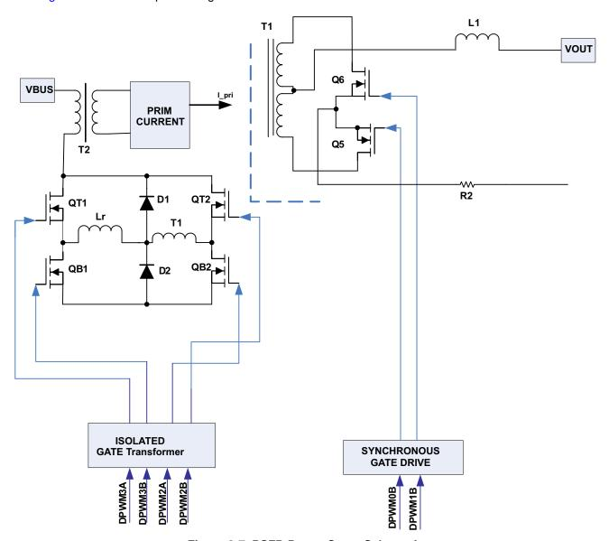
Figure 8-7. PSFB Power Stage Schematic
