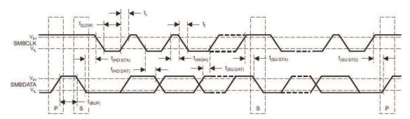
Figure 5-1. I<sup>2</sup>C/SMBus/PMBus Timing Diagram
