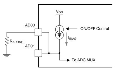
Figure 7-13. PMBus Address Detection Method
