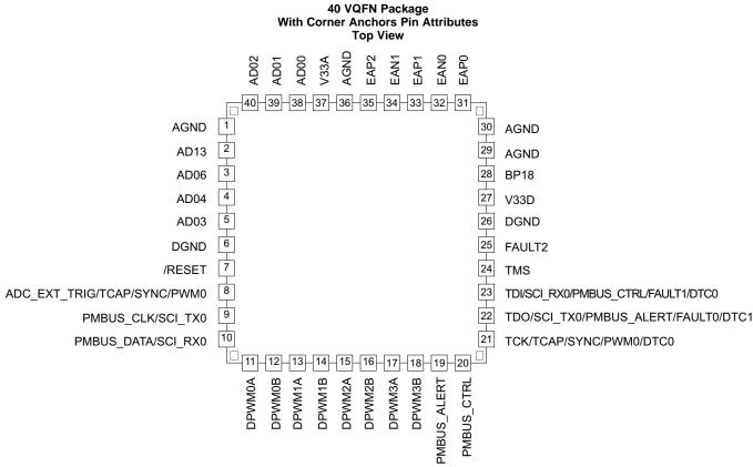
The RJA package has thicker package height compared to the RMH package. There are four corner pins on the RJA package. These features help to improve solder-joint reliability. The corner anchor pins and thermal pad should be soldered for robust mechanical performance and should be tied to the appropriate ground signal.
