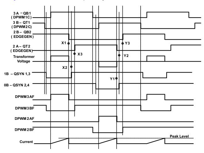
X1, X2, X3 and Y1, Y2, Y3 are sets of moving edges. All other edges are fixed
