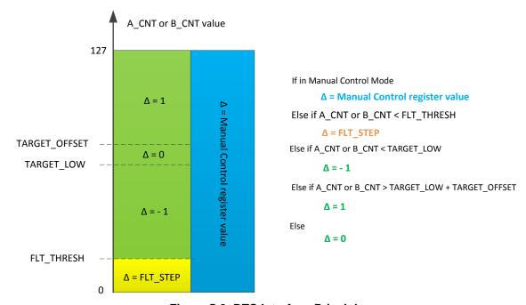
Figure 5-8. DTC Interface Principle
