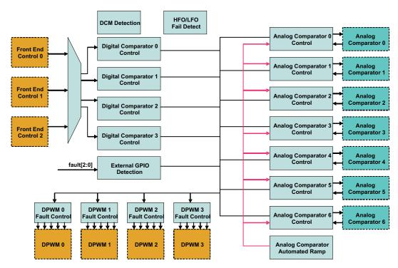
Figure 7-12. Fault Mux Block Diagram
