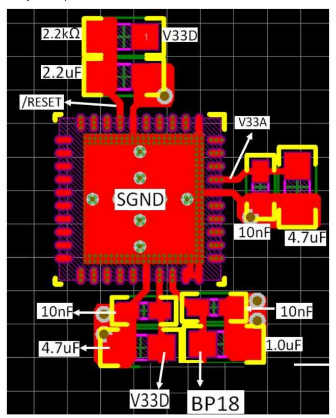
Figure 10-1. UCD3138A Layout Example
