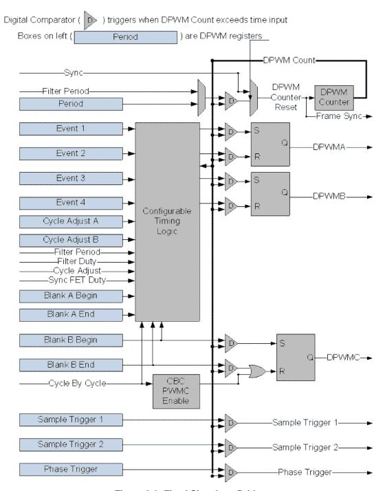
Figure 8-9. Fixed Signals to Bridge
