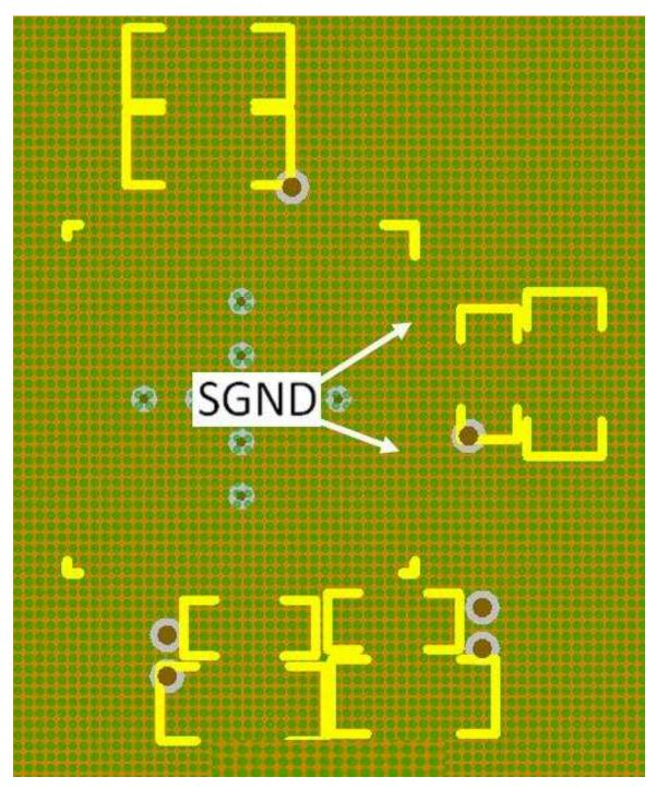
Figure 10-2. UCD3138A Layout Example, Internal Plane
