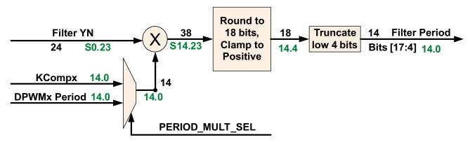
Figure 7-8. Final Section for the Filter
