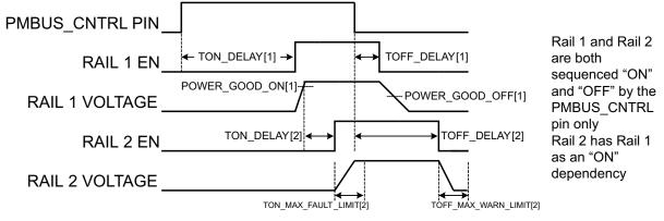
Figure 8. Sequence-on and Sequence-off Timing
