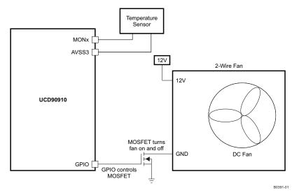
Figure 21. Two-Wire Fan Connection
