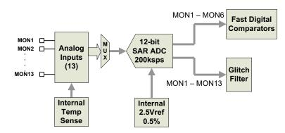
Figure 9. Monitoring Block Diagram
