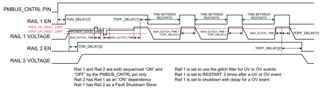
Figure 13. Sequencing and Fault-Response Timing
