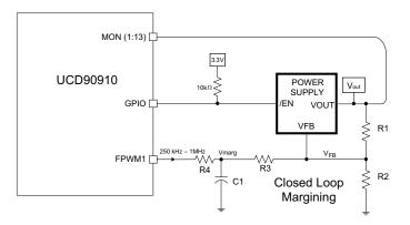
Figure 20. Closed-Loop Margining
