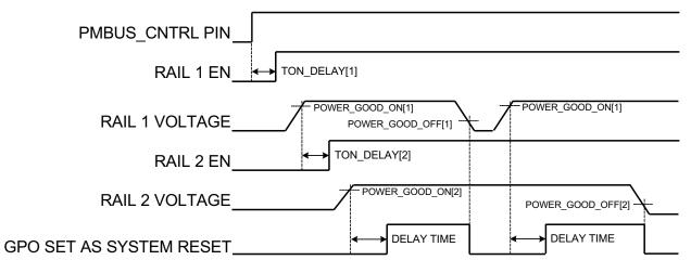
Figure 26. System Reset Timing Example
