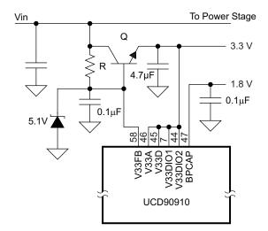
Figure 30. High-Voltage Supply With External Transistor
