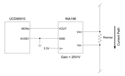
Figure 10. Current Monitoring Circuit Example Using the INA196
