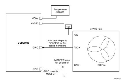
Figure 22. Three-Wire Fan Connection
