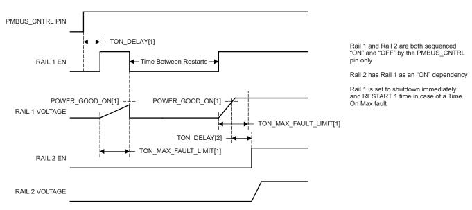
Figure 14. Maximum Turn-on Fault
