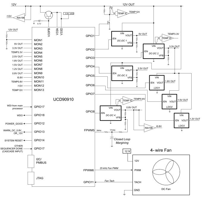
Figure 33. Typical Application Schematic
