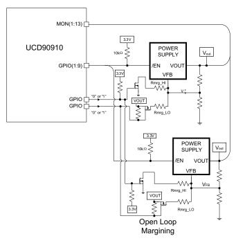
Figure 19. Open-Loop Margining
