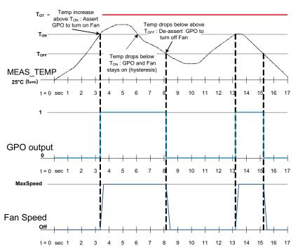
Figure 24. Hysteretic Temperature Control for 2- or 3-Wire Fans
