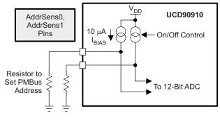
Figure 29. PMBus Address-Detection Method
