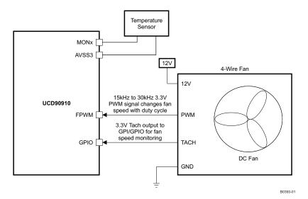
Figure 23. Four-Wire Fan Connection
