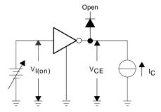
Figure 19. V<sub>I(on)</sub> Test Circuit
