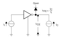
Figure 18.  $h_{fe}$  ,  $V_{CE(sat)}$  Test Circuit
