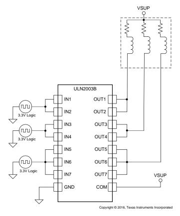
Figure 23. ULN2003B as Inductive Load Driver
