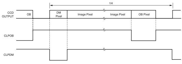
Figure 8. Timing for CLPOB and CLPDM
