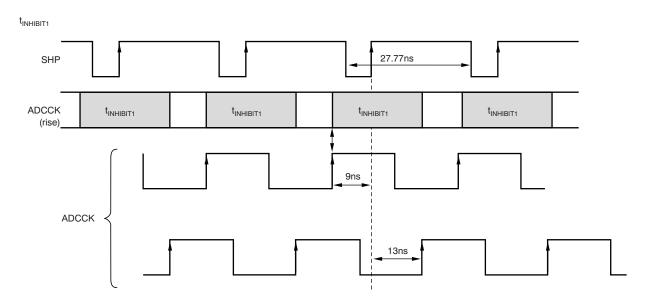
Note that in condition of OD (Output delay) = 00
