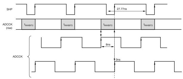
Figure 2. TG High-Speed Pulse Specifications (Detail of inhibit area)
