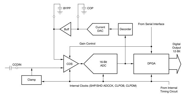
Figure 4. Simplified Block Diagram of VSP2582
