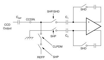
Figure 5. Block Diagram of CDS and Input Clamp
