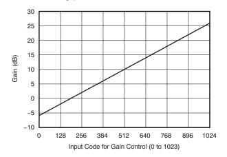
Figure 7. Setting Code vs. Digital Gain
