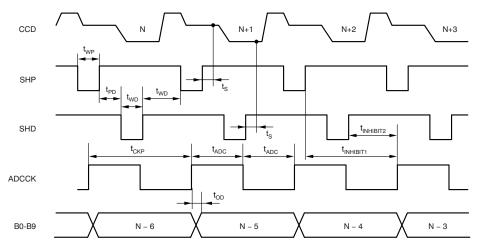
Figure 1. TG High-Speed Pulse Specifications
